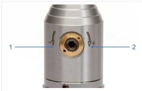
Fig. 2: Indication of the direction of rotation for clamping and unclamping the tool
