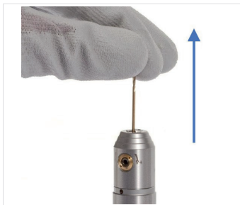
Fig. 7: Remove the tool
